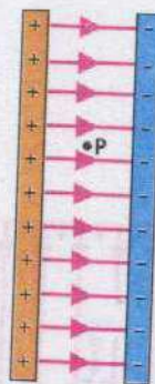
Fig. 12.19 The lines of force between the plates are normal to the plates and are directed from the positive plate towards the negative one.
