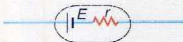
Fig. 13.18 An equivalent circuit of a cell of emf E and internal resistance r .
