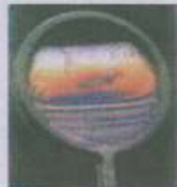
Fig. 9.5 Interference pattern produced by a thin soap film illuminated by white light.
