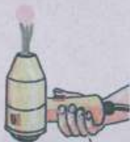
A table tennis ball can be made suspended in the stream of air coming from the nozzle of a test dryer.
